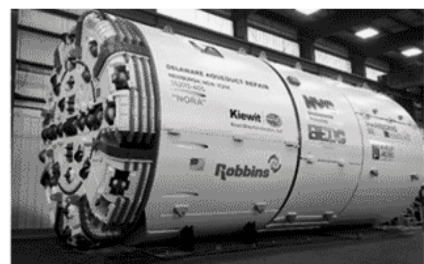
Delaware Aqueduct is 21.6 feet in diameter and weighs 2.7 million pounds.
